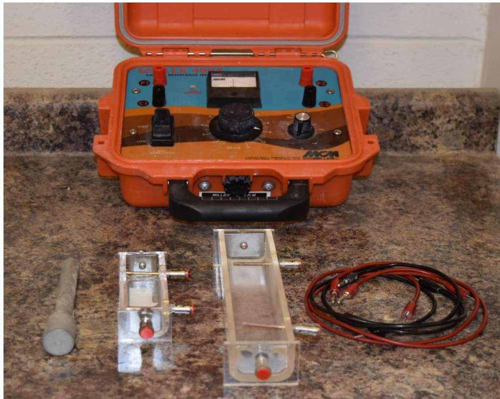
Electrical Resistivity Meter with Molds and Hammer
